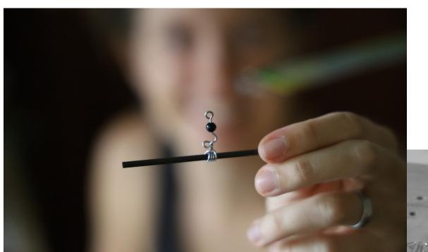
Shown left: half of a handmade jewel-bearing swivel made from stainless steel, onyx and carbon fiber.
